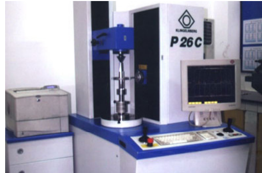
P26C gear measuring center Klingelberg GmbH, Germany
