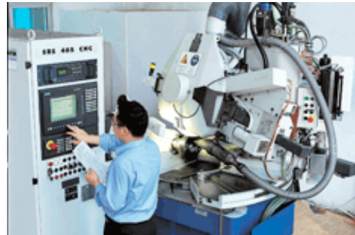
SRS405-CNC shaver grinder Gleason-Hurth, Germany (9-axis)
