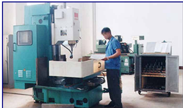
Jig Boring and Milling Machine
