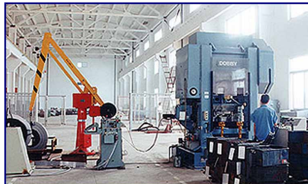
High-speed Punching Machine 80 Ton YAMADA, Japan
